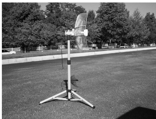
Figure 1.11 A Parabolic Antenna Isn't Good for WarDriving
