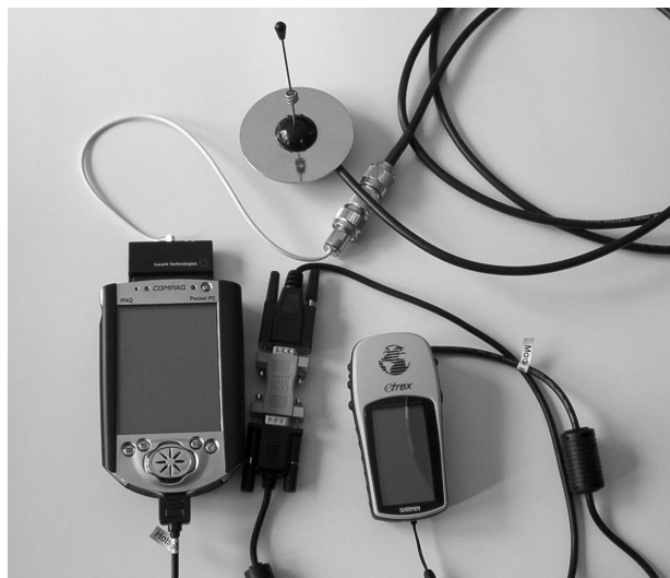
Figure 1.6 A Typical PDA WarDriving Setup
