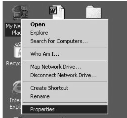
Figure 1.20 Disabling the TCP/IP Stack Step One
